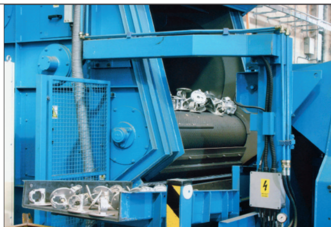
Fig. 9 Granigliatrice a Tappeto Rampante® in gomma modello SG8 RCH. Shot Blast machine Tappeto Rampante®, with rubber belt conveyor, model SG8 RCH.
