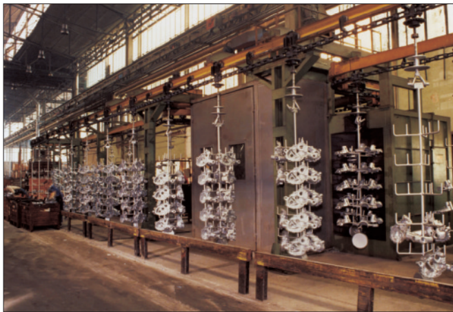
Fig. 7 Granigliatrice a gancio a giostra modello Sandermatic 7. Tunnel type shot blast machine with hook trolleys model Sandermatic 7.
