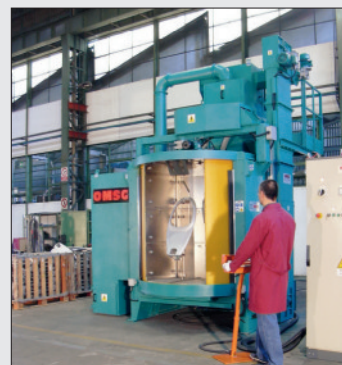
Fig. 5 Granigliatrice a revolver modello REV 6/12 M FAC. Revolver-type shot blast machine model REV 6/12 M FAC.
