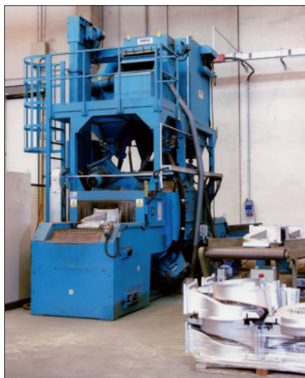
Fig. 3 Granigliatrice a nastro in rete modello CWB 850. Shot blast machine with endless wire mesh conveyor model CWB 850 4/FAC.
