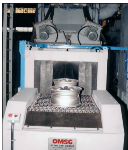
Fig. 8 Granigliatrice a nastro in rete modello CWB 850 8T. Shot blast machine with endless wire mesh conveyor model CWB 850 8T
