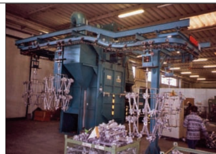
Fig. 4 Granigliatrice a gancio, a giostra modello Sandermatic 5 E. Tunnel type shot blast machine with hook trolleys model Sandermatic 5 E.
